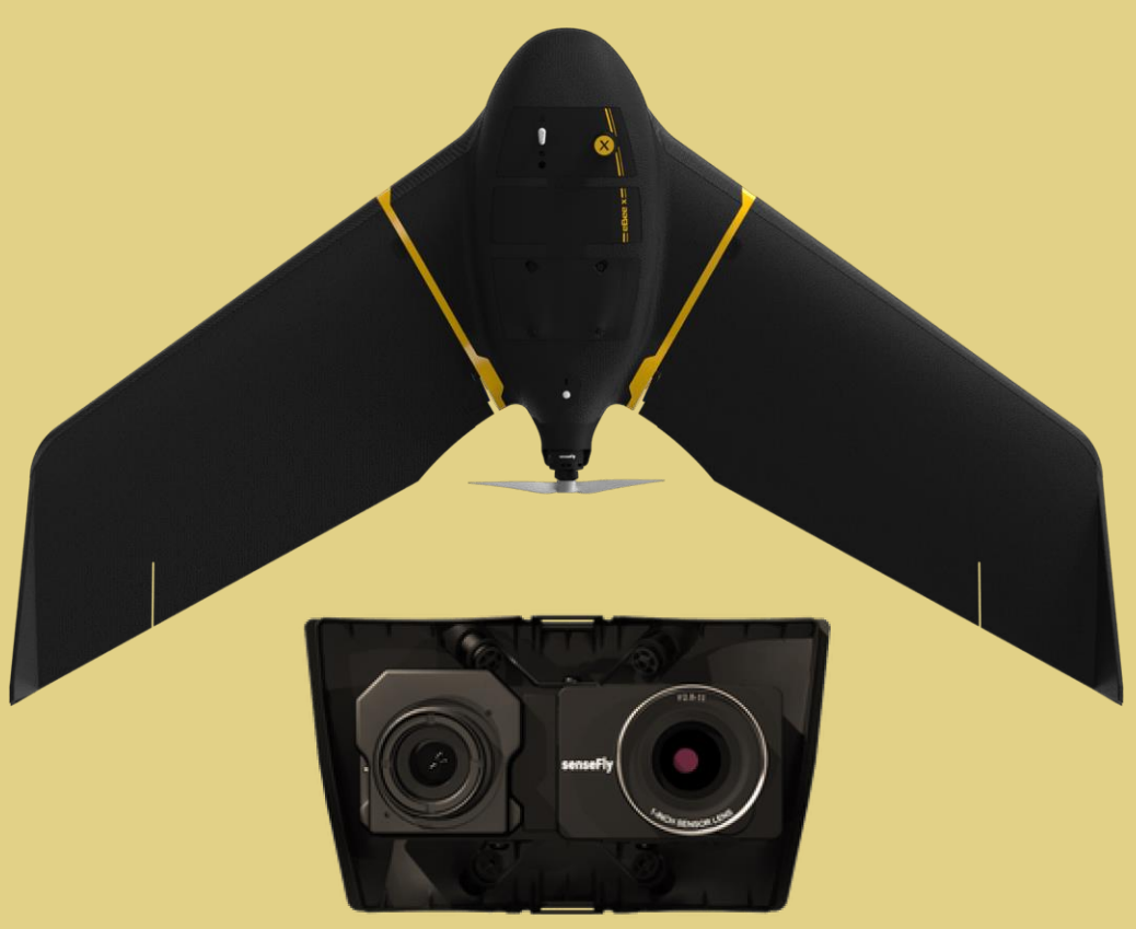
Figure 1: eBee X drone and Duet T Camera (AgEagle Aerial Systems, Inc.)
