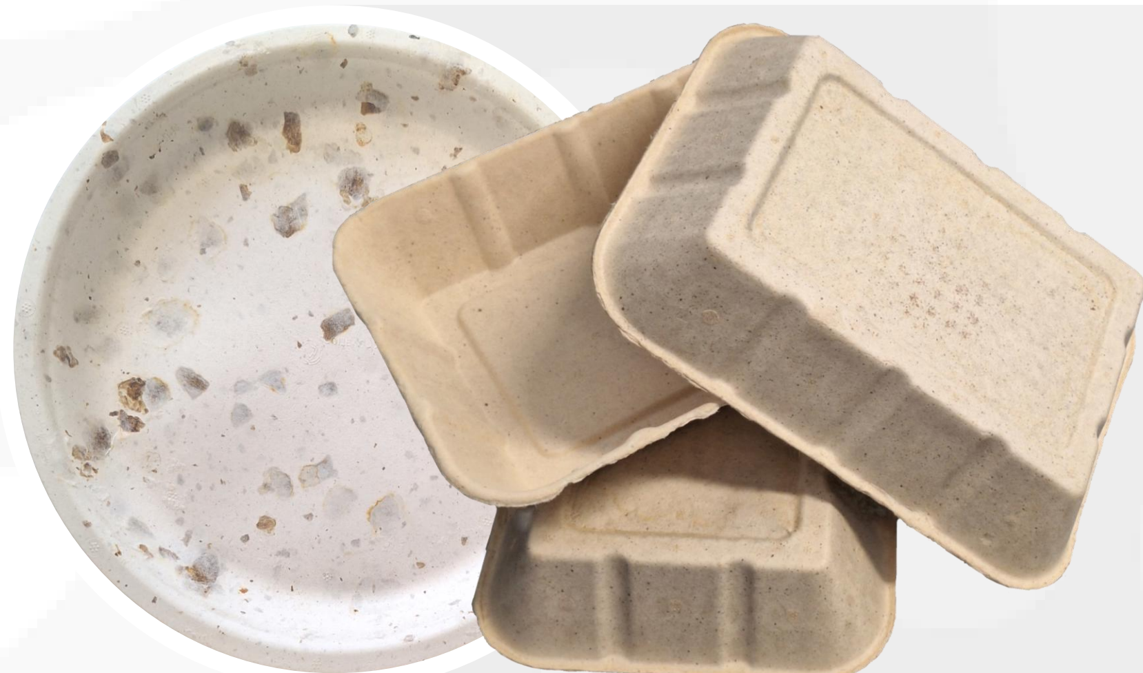
Molded trays containing 25% tubers and molded plates containing 10% peels, produced using a TMP-based formulation.
